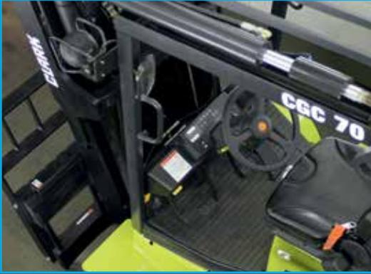
The interior of the generously designed operator's workplace offers the driver sufficient headroom and legroom. The driver can enter and exit comfortably via a large step. Handles on both sides of the truck increase safety. The steering column is tiltable and can be adjusted individually.
