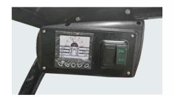
Interactive instrument: The instrument adopts LCD display with four interactive buttons, and has one CAN bus communication function. The communication protocol is compatible with CANopen and SAE |1939 standards.
