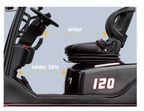
The extra foot space is provided to reduce operator fatigue significantly. The new wide-open, non-slip step makes getting in and out easy and safe.
