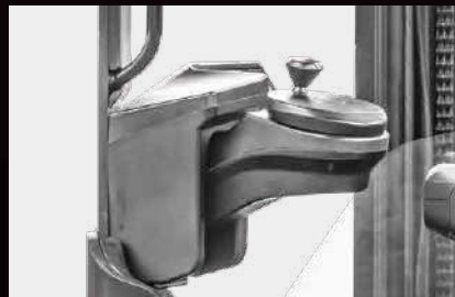
Steering wheel position can also be adjusted
