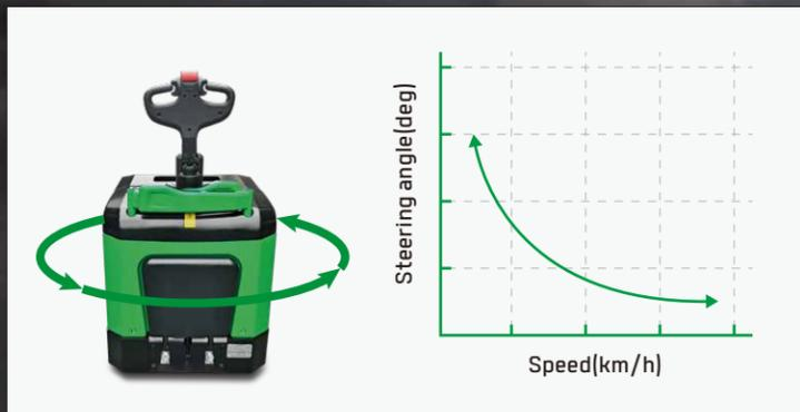
A standard feature of automatic speed decrease along with the steering angle increase is provided.
