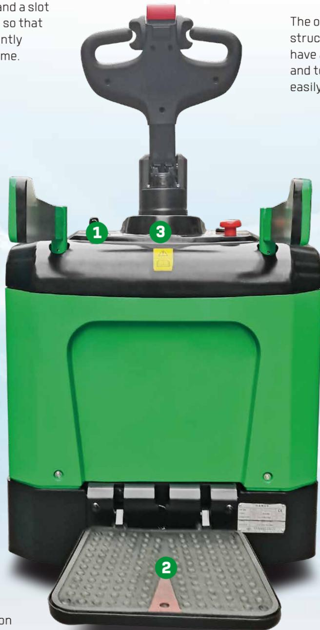
The battery box cover is designed with an air spring to allow the cover to be opened more easily.
